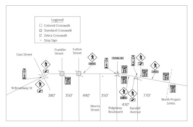
Figure 16: Existing Broadway Street Signing and Pavement Markings
